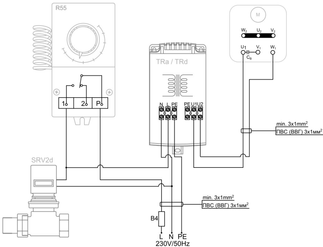
Thermostat R55 controls the operation of SRV2d valve and TRa/TRd speed regulator. TRa/TRd allows for 5-step fan air flow switch.
