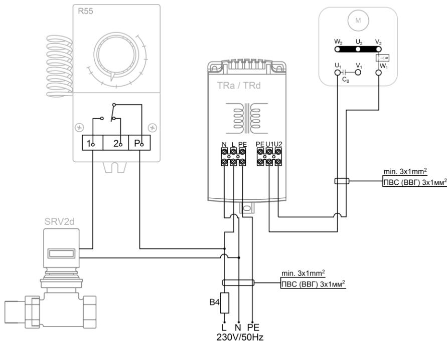
Thermostat R55 controls the operation of SRV2d valve. TRa/TRd speed regulator allows for 5-step fan air flow switch.
